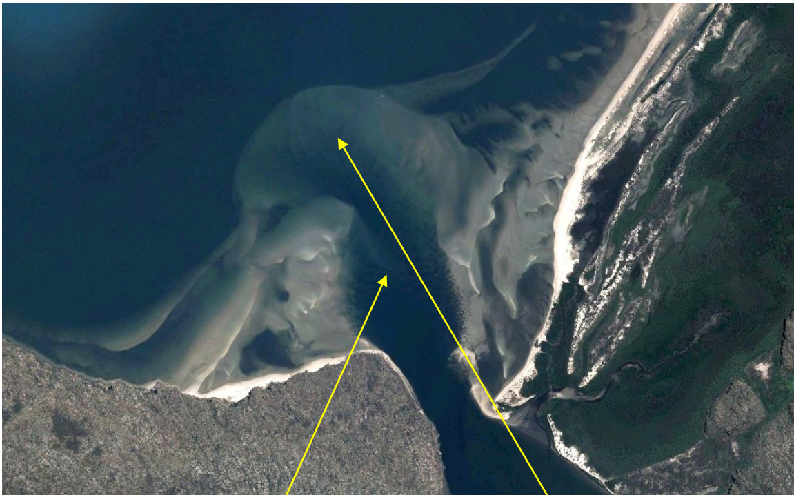
Figure 1. Sand shoals clearly visible outside the entrance to KGR. Note the channel cut through the shoals by the tide. The shallowest part of the channel is usually at the seaward end of the channel.
